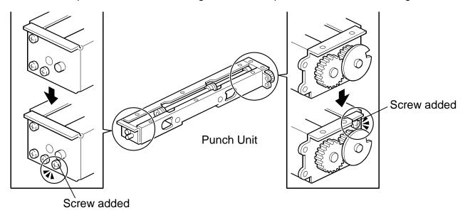
Due to the above punch unit modification, the screw position of the punch drive bracket have been changed. The length of the oval hole in the punch drive bracket has been changed from 8 mm to 12 mm.
